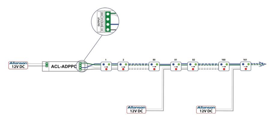
Each Allanson 60W Power Supply (CV125 series) can run maximum 80 modules. Each ACL-ADPPC can run 8-360 modules.
